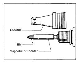
To install the bit, follow the removal procedures in reverse.
